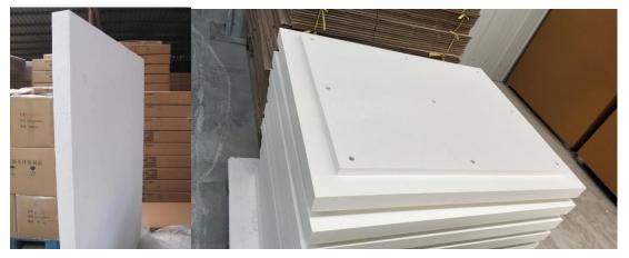
The ceramic fiber board is refined by vacuum forming process, dried and machined. In addition to the excellent performance of the corresponding bulk aluminum silicate fiber cotton, various types of ceramic fiberboards have hard texture, excellent toughness and strength, and excellent wind erosion resistance.
